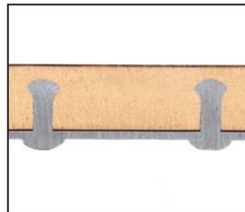
**Tamper proof expansion rivets** secure frame onto sturdy MDF (Medium Density Fiberboard) core. 32% more holding power than screws and particleboard.
